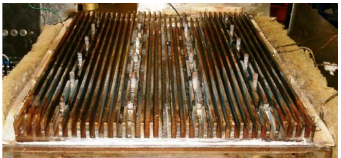
Finned heatsink is bolted to the bottom of the water reservoir. This heatsink is a key performance component, as it significantly increases the heat transfer area and helps cool the flue gases.
