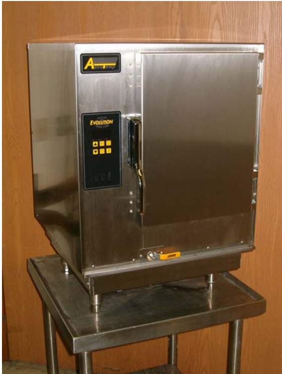
Front view. Drip tray is one-piece, fixed and spans the entire front face.
