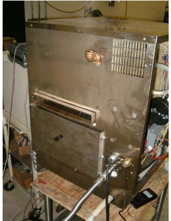
Rear view, with the flue above a heat shield on the left and the electric, gas and water connections on the right.
